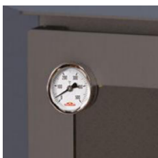
Oven with 500 °C thermometer to monitor temperature.
